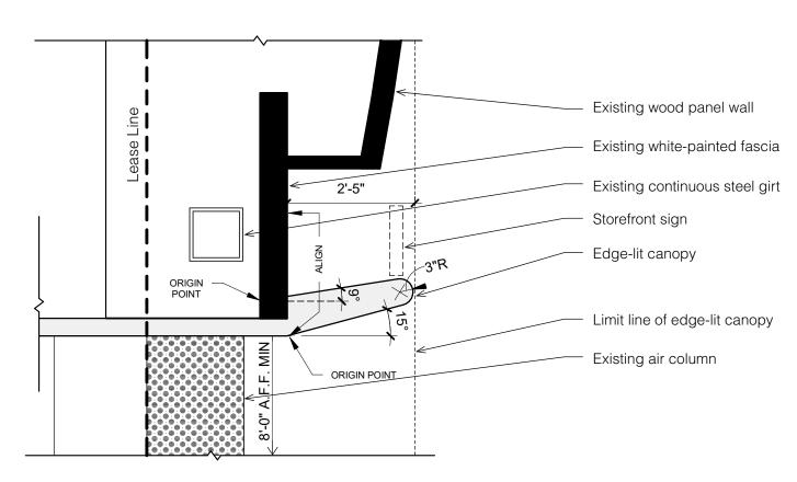
Terminal B In-Line Concession Canopy Section - Low Soffit Condition
